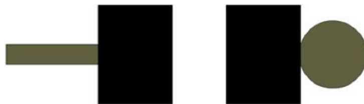
Figure 6, Example of bad SM pad to via spacing
